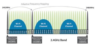
Note: Channels 37, 38, and 39 are used with the Bridge.
