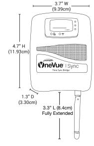
Note: Orient the Bluetooth Antenna to point straight down (vertically) from the device to maximize its signal reception.
